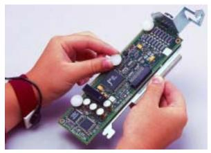
4. Slide the hook near the bottom of the circuit board mounting bracket into the support slot on the main control board.
